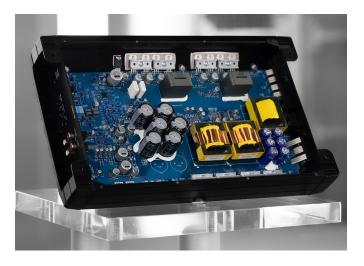
**Simplified Installation** – The amplifier was intentionally designed with sound controls located on the side panels, instead of the top panel, making it easier to access gain and crossover controls when installed under vehicle seats or in shallow-depth locations. Removable end caps were added to cover the side controls and connections, providing a clean, sleek finish to the amplifier.
